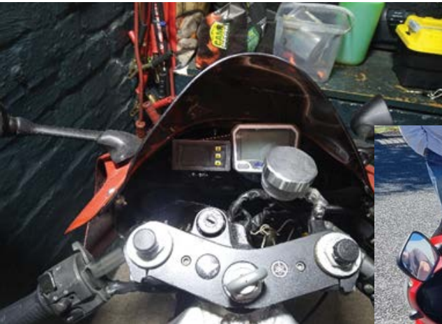
Gauges mounted under screen
