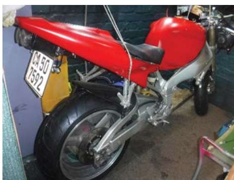
Rolling Chassis ready for motor
