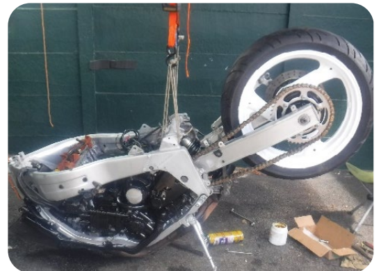
Then rebuild rear shock & swingarm
