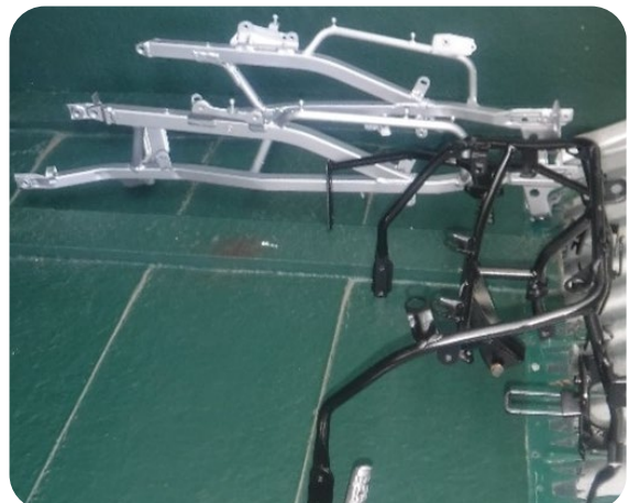
Respray all the sub-frames
