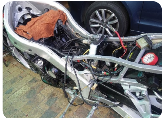
Rewiring the loom and electrics
